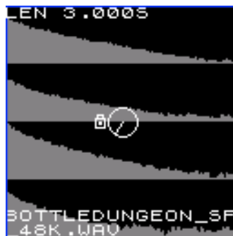
Illustration 3: A locked knob will display a lock, and the orientation you should turn the knob towards to unlock it.
