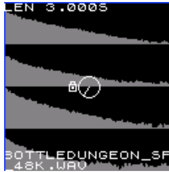
Illustration 5: A locked knob will display a lock, and the orientation you should turn the knob towards to unlock it.
