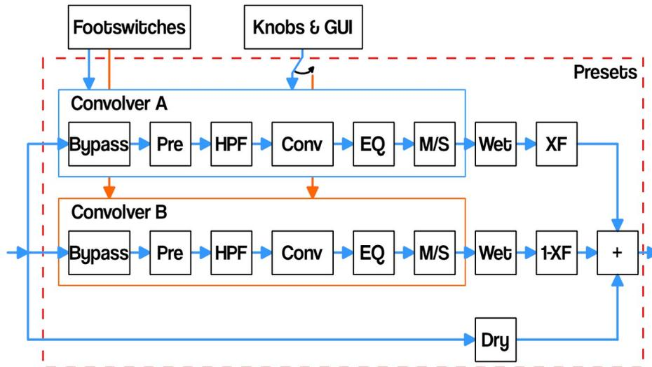
As you can see the two internal convolvers both have their own processing chain: PRE for predelay, a high-pass filter, 4-band parametric EQ and followed by a Mid-Side matrix (aka stereo width on the front panel).
