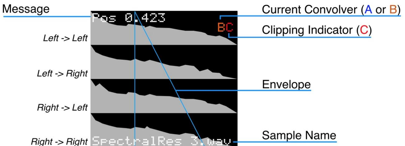
If a plain stereo sample is loaded instead of a 4 channel sample, only two channels are visible. Why these 4 channels? This is for the so-called stereo matrix. The left input can also influence the right output and vice versa.
